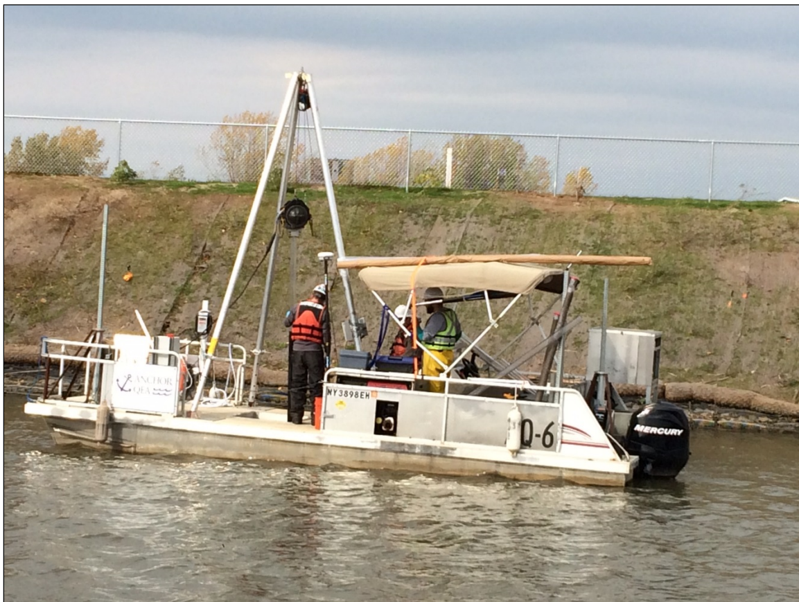
Geotechnical Sampling in a Confidential River (Photo courtesy of Anchor QEA, LLC)
